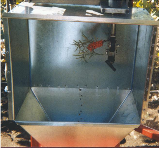
**Fig. 2. Mechanism to shake the severed sea buckthorn branches in the vertical direction. As the berries became detached, they were collected in a plastic bag located at the bottom of the hopper.**
